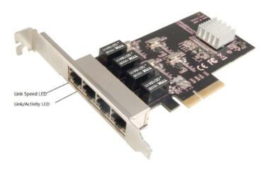
There are two LEDs at the two bottom corners of each of the Ethernet port on the network card.
