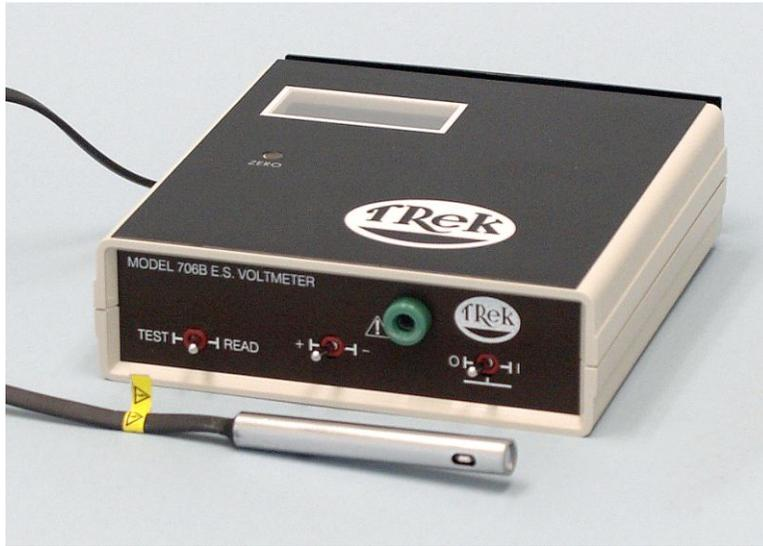
The Trek Model 706B portable electrostatic voltmeter is designed to perform highly accurate noncontacting surface electrostatic voltage measurements. Applications include measurement of photoreceptor surfaces in copiers and laser printers.
