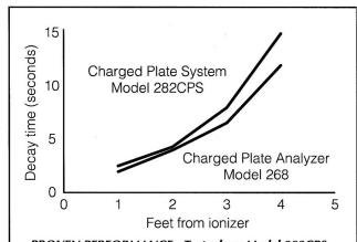
**PROVEN PERFORMANCE - Tests show Model 282CPS** decay-rate measurement accuracy correlates closely with that of the ME Model 268 charged plate analyzerwhich meets ESD Association Standard No. 3.
